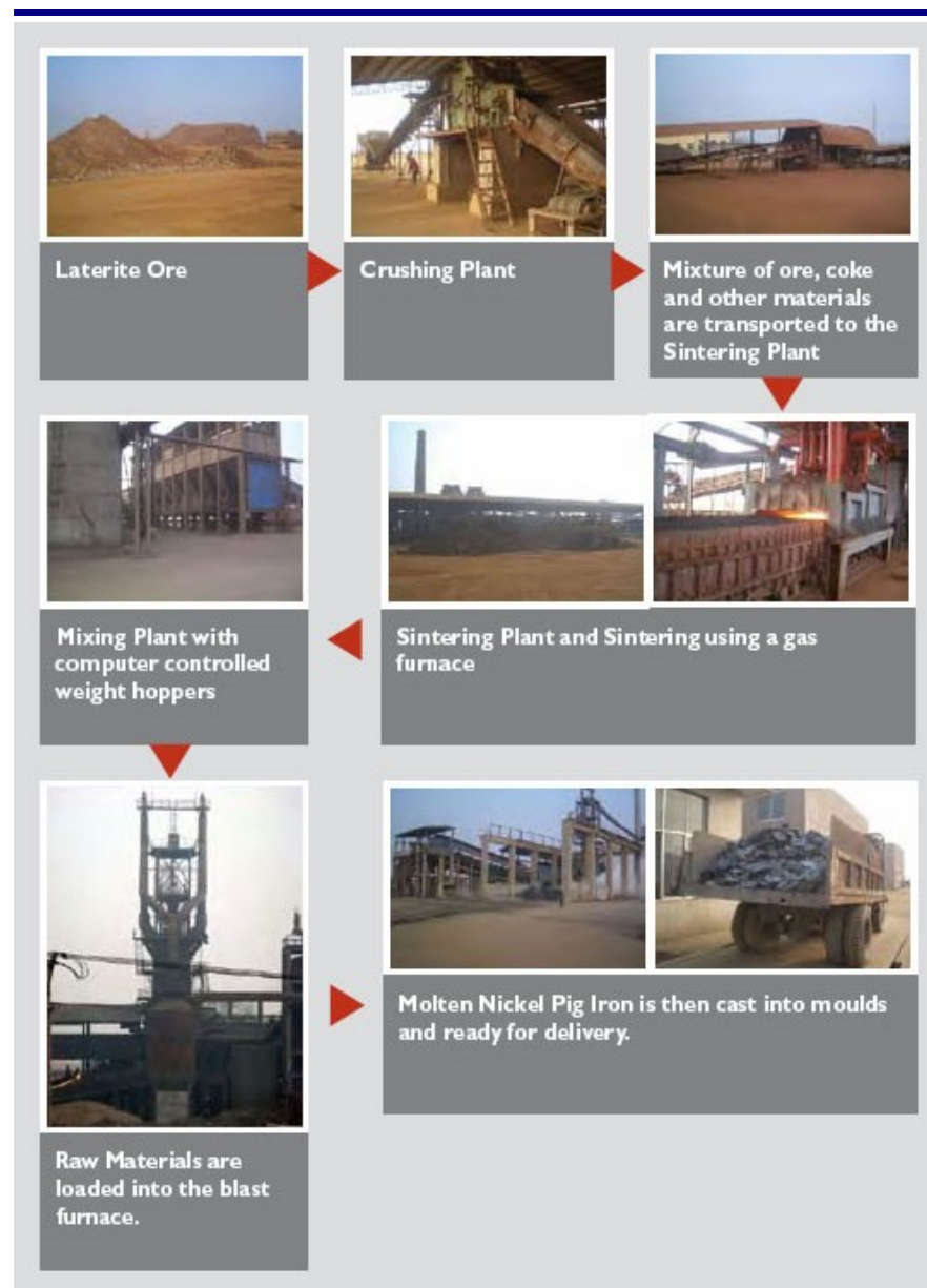
Fig 17: NPI production process
